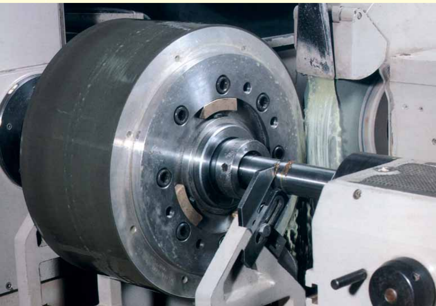
Truing of resin bonded centerless wheel
